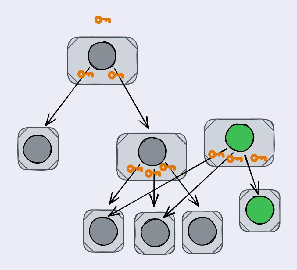
The next revision of a block is encrypted with essentially a hash of the current revision's key
